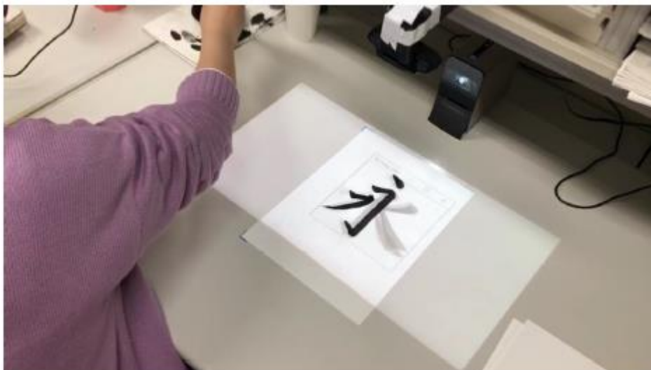
Figure 2.9: The interface of calligraphy training system using projection mapping
