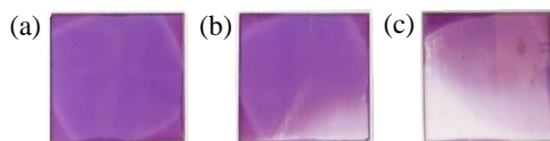
Figure 3.6 The samples rubbed by auto-rubbing: (a) unrubbed, (b) 0.63 kN/m 2 -rubbed and (c) 2.51 kN/m 2 -rubbed samples. Sample size: 2.5 cm × 2.5 cm.
