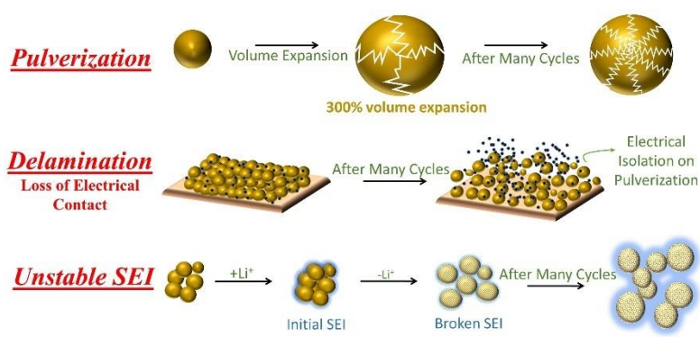
Figure 4: Drawbacks associated with Si anodes
