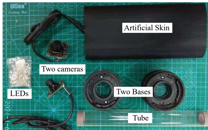
Figure 3.3: The main components for building the TacLINK.
