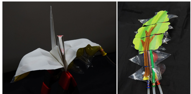
Figure 9: Flying crane with one xBalloon actuator (left), and swaying tree with three xBalloon actuators (right).
