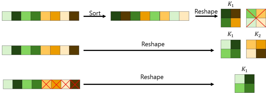
Fig. 1. Conventional filter pruning (top), the actual involution kernel (middle), and the diet operation (bottom). The green and brown indicates different kernels and K_i stands for the i -th kernel. If the results are different from the middle, the spatial information is lost. Conventional pruning sorts the weights before reshaping therefore the result differs from the actual kernel. Diet in contrast prunes the weights before reshaping therefore the results are equal to the actual kernel.
