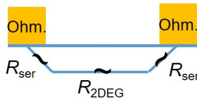
Figure 4.14: The measured TLM resistance can be consider as a series of resistors.
