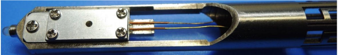
Fig. 15. Specimen holder for Hitachi S-5200Tip of the specimen holder for Hitachi S-5200.
