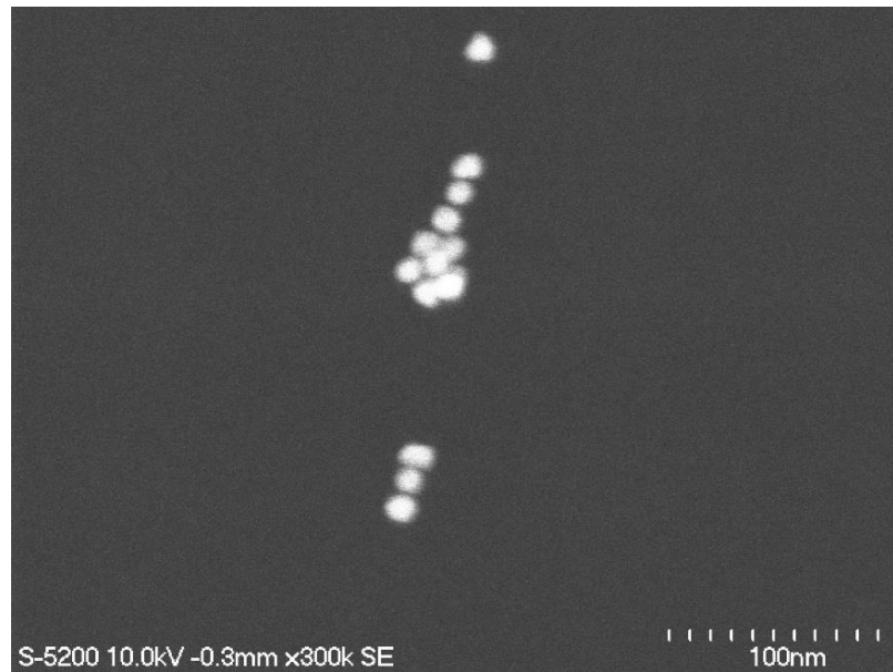
Fig. 21. SEM image of gold particles on the top of grid (in vacuum), and on the rear of grid (in water).
