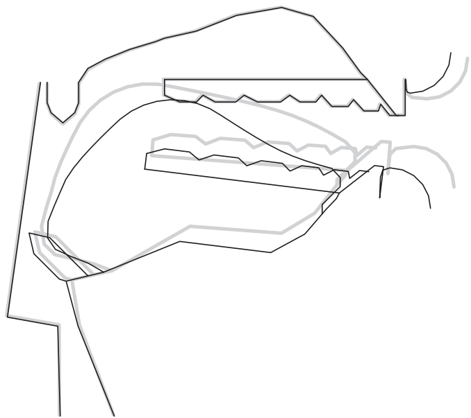
Figure 2: Midsagittal shapes of the vocal tract model for the vowel /a/ with normal (standard) articulation (gray lines) and Lombard articulation (black lines).
