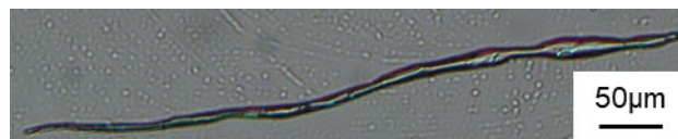
Fig. 3. An optical microscopy image of a PVA fiber.
