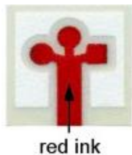
Figure 1.1 Patterned paper, or so-called microfluidic paper-based analytical device ( \mu PAD), after absorbing Waterman red ink (5 \mu L) by capillary action. Adapted with permission from ref. 2. Copyright © 2007 WILEY - VCH Verlag GmbH & Co. KGaA, Weinheim.
