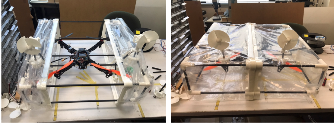
Fig. 2. A hybrid vehicle prototype in UAV mode (left) and USV mode (right).
