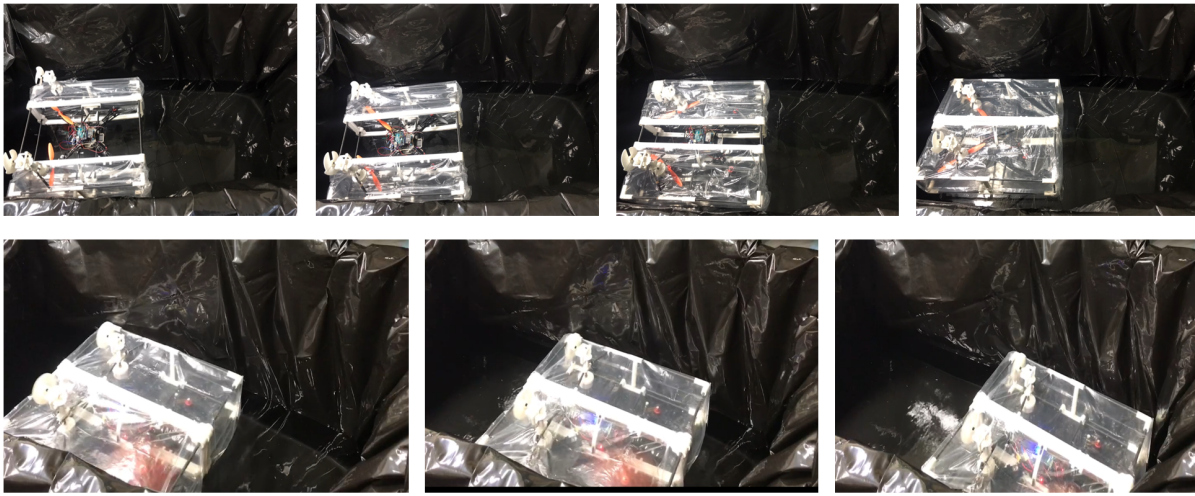
Fig. 8. Vehicle mode transition and movement test in a laboratory testbed: (top) snapshots of the transition from the UAV mode to the USV mode, (bottom) the USV mode moving on the water surface.
