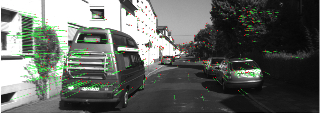
Figure 2.3: Motion estimation of the feature in the image [3]
