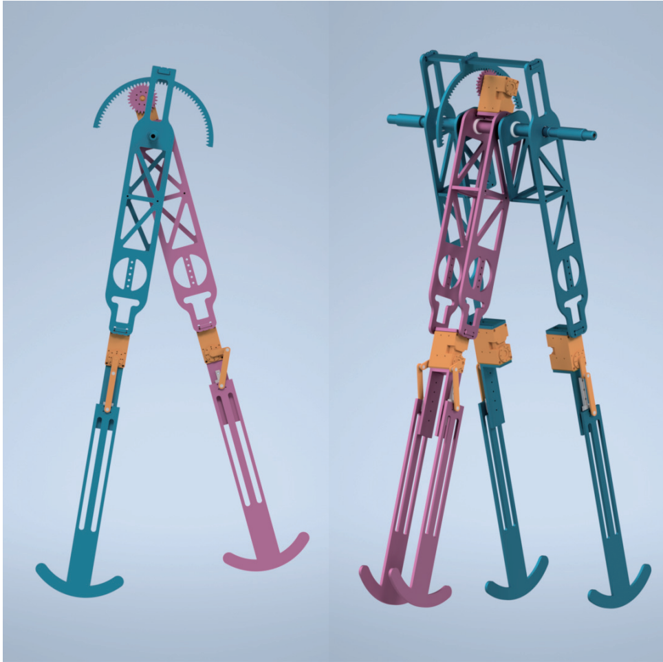
Figure 7.8: CAD of a compass bipedal walking robot designed to conform to the simulation style
