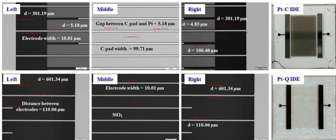
Figure 2. Optical microscope images of different parts from fabricated IDEs with geometry measurement and photograph of Pt-C IDE and Pt-Q IDE.
