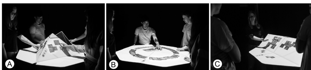
Fig. 4.7 KirigamiTable: Designing for Proxemic Transitions with a Shape-Changing Tabletop [114]. The table performs the following transformations - four-fold (A), flat-fold (B) and two-fold (C)
