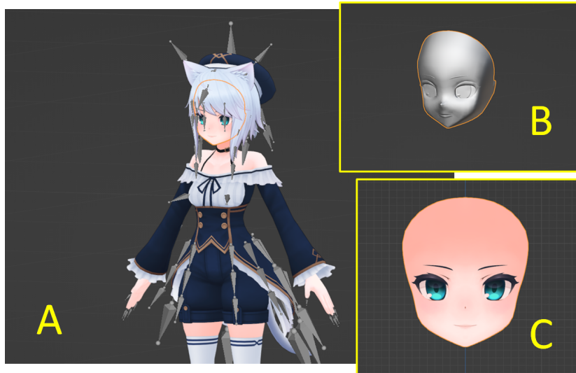
Figure 3.2: The image of data extraction of the training data. Complete avatar data was load in Blender GUI (A). This image shows the extraction of facial parts. facial mesh was separated and saved as another mesh data file (B). Facial texture was obtained as orthogonal rendering result (C).
