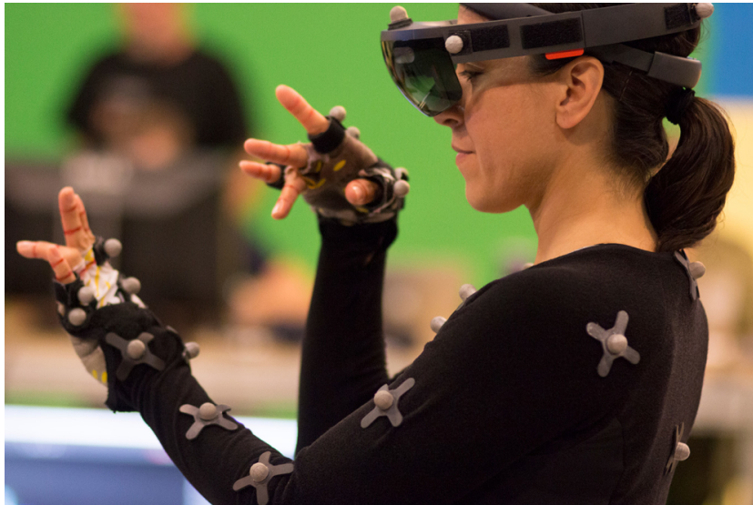
Figure 2.9: VICON, a dedicated motion tracking system. It uses a suit filled with markers and camera system. http://www.vicon.jp/
