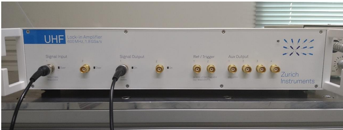
Figure 3.21 UHF Lock-in Amplifier from Zurich Instruments used during the noise measurements.
