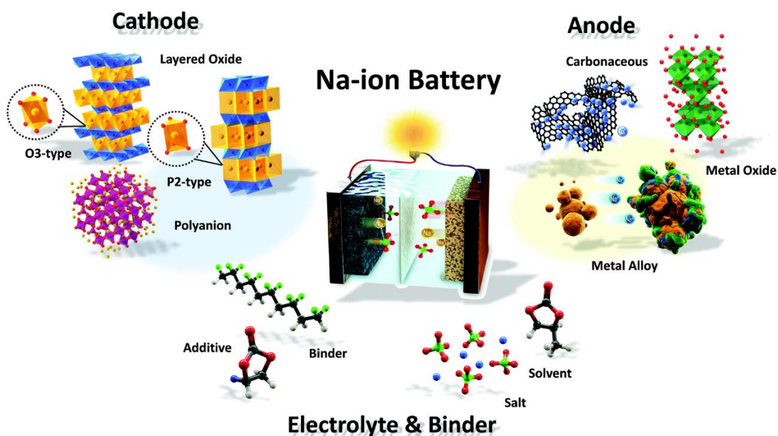
Figure 13: Illustration of SIB components and battery system 85 .
