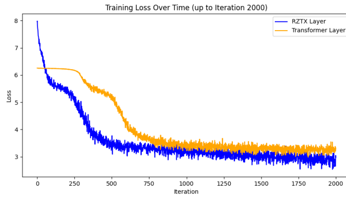
Figure 3.14: The loss variation over the first 2000 iterations when using the RZTX layer and the standard transformer layer.
