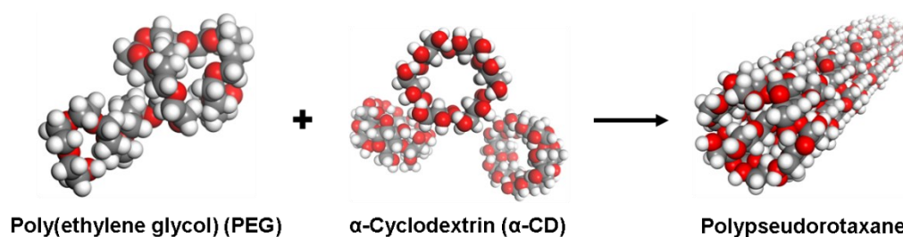
Fig. 1.4 The model of polypseudorotaxane consisting of poly(ethylene glycol) and \alpha -cyclodextrin.
