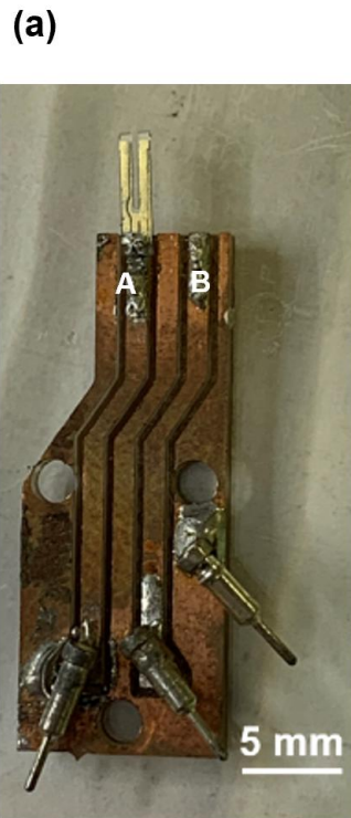
Fig. 4.4.(a) A tuning fork is soldered on a fabricated PCB. Position A and position B are connected by a gold wire. (b) The PCB is stuck to a small aluminum bulk.
