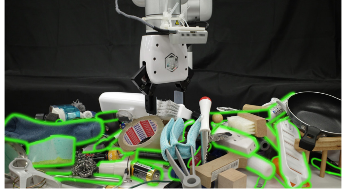
Fig. 1. Common grasping methods on the densely cluttered table: they require analyzing all objects in the scene (some of which are highlighted with a green border), which introduces significant computational redundancy and weakens the analysis of the object to be grasped. Additionally, their reliance on a fixed view often leads to incomplete object geometry at the view boundary.
