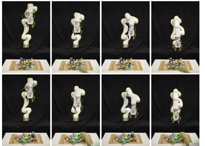
Fig. 15. Cases of the DRD process under hand dynamic interference. Each row corresponds to one case, and the images in each row respectively illustrate the initial approach of the robot to the target object, the first deviation of the robot after interference, the re-approach (return) of the robot to the target object after the hand departs, and the second deviation of the robot after the second interference. Yellow, green, and blue borders are also used to highlight the robot, the human hand, and the target objects, respectively.
