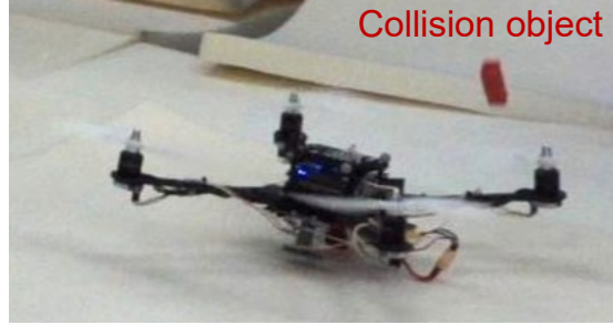
Figure 4.20: The real-flight collision experiment is performed by freely dropping an impact object into the propeller's rotation zone while the quadrotor is flight.
