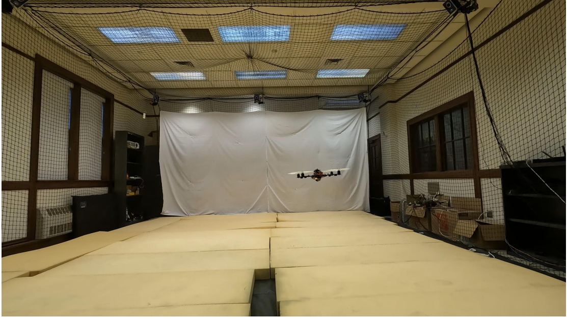
Figure 3.7: Flight experiment setup for the Tombo quadrotor: The quadrotor’s position is tracked using Vicon cameras and processed by a ground computer, which transmits the data to the onboard Pixhawk 6X flight controller via the MAVProxy protocol. The Pixhawk 6X then computes the position error between the desired and actual locations and generates the corresponding PWM percentage commands to the motors.
