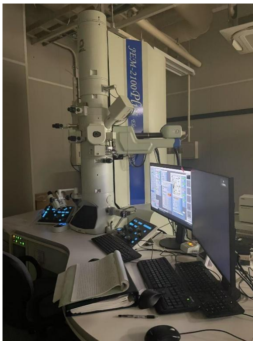
Figure 2.1 the photograph of TEM-2100plus
