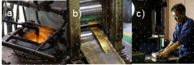
Figure 2.a) Melt the metal. b) Rolling the alloy block to reduce thickness. c) Harming progress for Kanazawa gold leaf.
