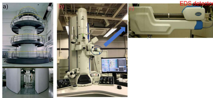
Figure 28. a) is Hitachi H-3000 TEM form Osaka university; b) is the JEM-2100Plus TEM with an eds detector; c) is the eds detector
