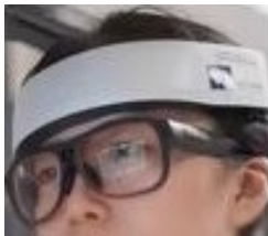
Figure 3.5: Participant wearing measurement devices. Displays the setup of eye-tracking glasses and the fNIRS device during data collection.
