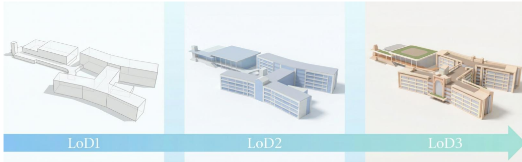
Figure 1.1: Models with different levels of detail. LoD1 represents coarse massing, LoD2 provides intermediate structural definition, and LoD3 captures detailed architectural representation.
