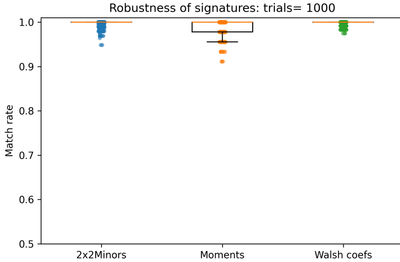
Figure 4.3: Distribution of match rates between Theoretical and Synthetic signatures under 1000 random parameter perturbations. The result shows structural invariance over parameter perturbation especially of 2 \times 2 Minors ( i_1, \dots, i_{13} ) and Walsh coefficients ( e_0, \dots, e_{123} ).
