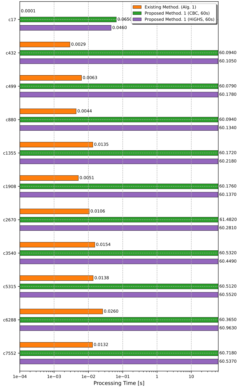
Figure 3.7. Runtime comparison (seconds) for Proposed Method 1 (Cbc/HiGHS, 60 s) and heuristic across ISCAS-85 benchmarks. Timeout at 60 s shown for unsolved instances.
