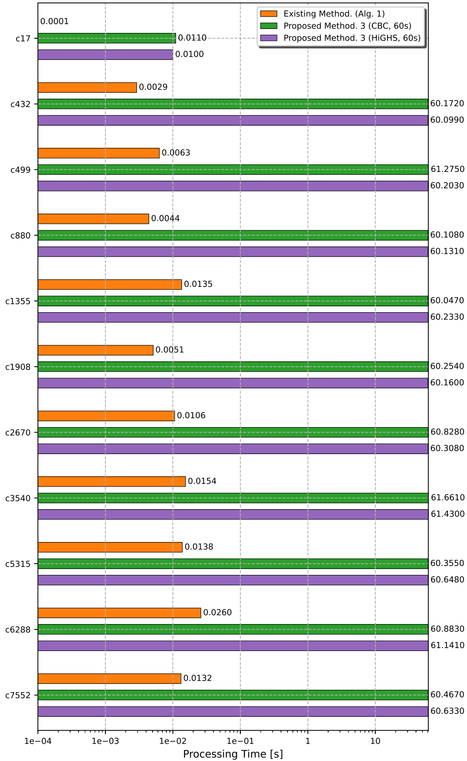
Figure 5.3. Runtime comparison (seconds) for Proposed Method 3 (Cbc/HiGHS, 60 s) and heuristic across ISCAS-85 benchmarks. Timeout at 60 s shown for unsolved instances.
