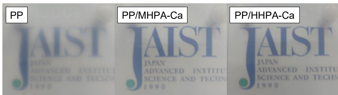
FIGURE 2.13 Photographs of injection-molded plates with 1 mm thickness.
