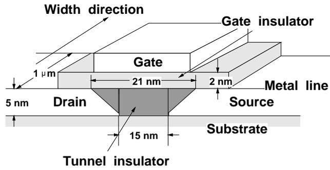
Figure 1. Schematic view of structure of metal/insulator tunnel transistor (MITT).
