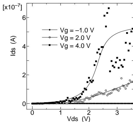
Figure 5. I-V characteristics of MITT.
