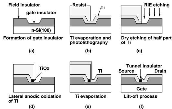
Figure 3. Fabrication process of MITT.
