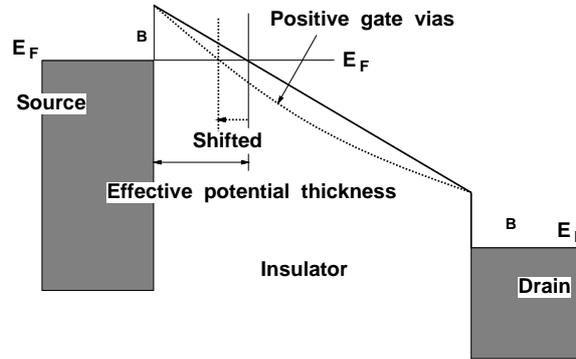
Figure 2. Energy band diagram of source/tunnel insulator/drain in the MITT.
