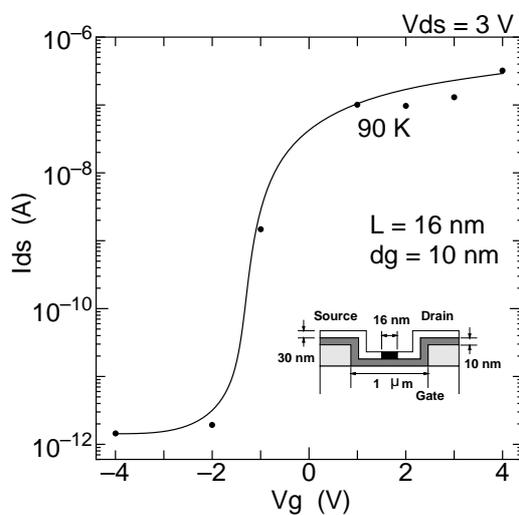
Figure 4. Experimentally obtained transfer characteristics of MITT at 90 K.
