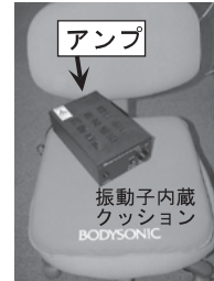
図3 Bodysonic 言語学習用システム JX-1 Fig. 3 Bodysonic JX-1 system for training of English speech/listening.
