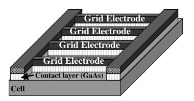
Electrode is removed from the cell by etching the GaAs contact layer.
