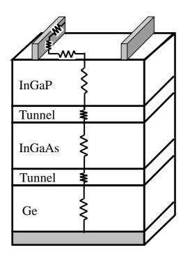
Electrode resistance ( $R_{SE}$ ) Contact resistance Lateral resistance ( $R_{SL}$ ) Layer (InGaP) resistance Tunnel resistance ( $R_{T1}$ ) Layer (InGaAs) resistance Tunnel resistance ( $R_{T2}$ ) Ge substrate resistance
