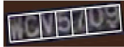
Fig. 2. Failed character segmentation resulting in some regions having more than one characters enclosed. This usually leads to recognition errors.
