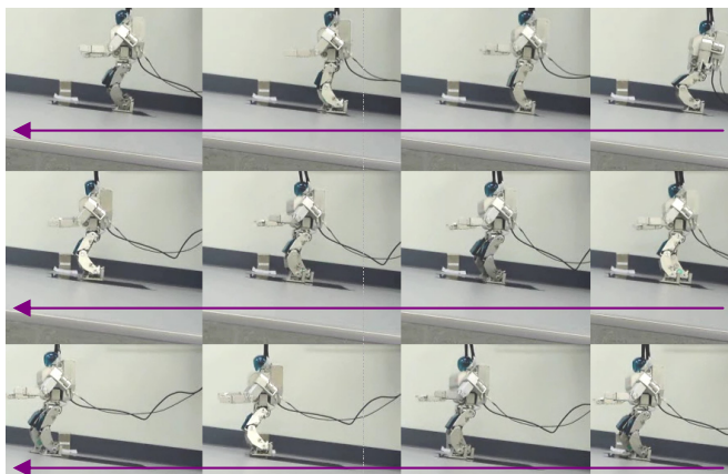
Fig. 17 Snap shots of a 6-degree uphill walking
