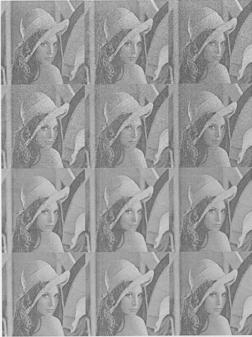
Figure 3: The resulting halftone images and the restored images: Top row , Ordered Dither, Error Diffusion(Floyd and Steinberg), and the halftone image by 1-flip(DBS). Second row , the halftone images by 4-flip, 9-flip, and 16-flip. Third row , Original image, the restored image of Error Diffusion, and that of 1-flip. Bottom row , the restored images of 4-lip, 9-flip, and 16-flip.
