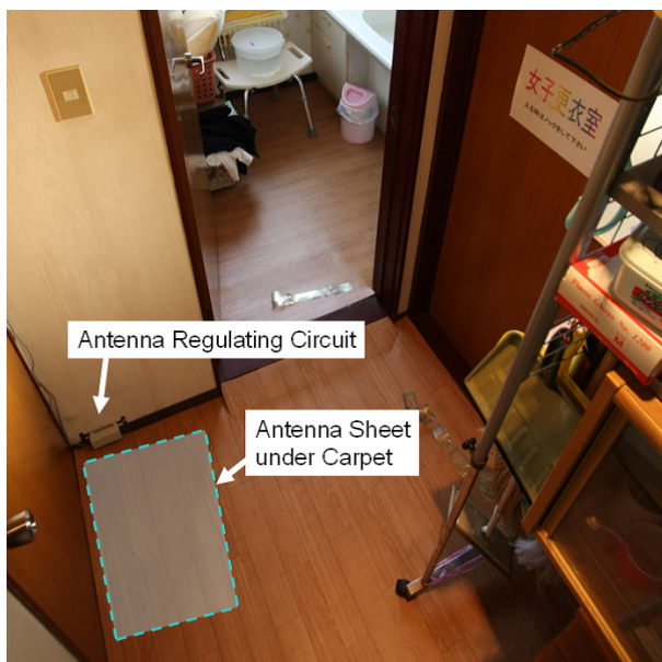
Figure 11. Deployment of an antenna in front of a restroom (No. 2 antenna in Figure 5).
