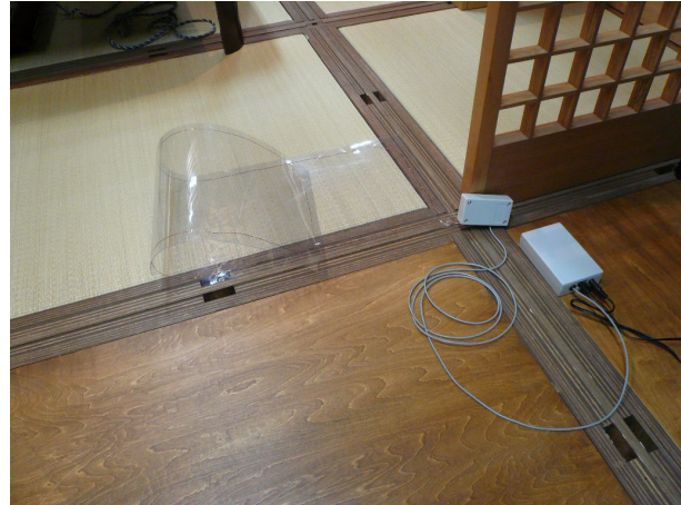
Figure 1. RFID antenna sheet, regulation circuit box, and reader box.
