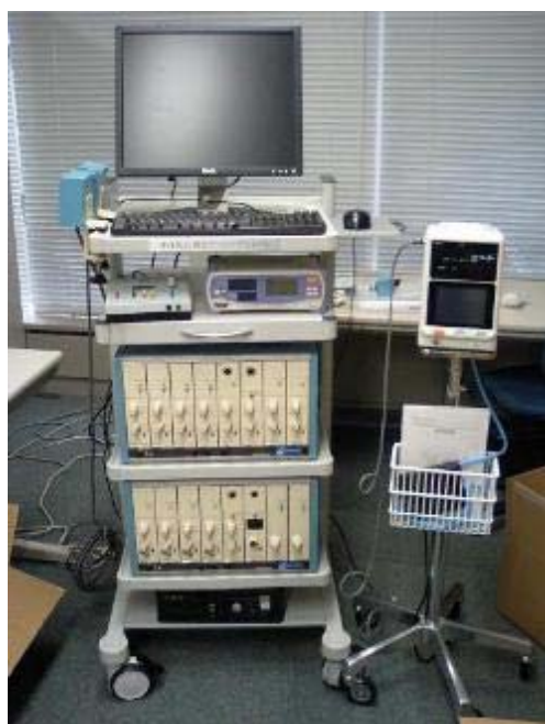
図5.3 Multi-Physiological Information Measuring System (MPIMS)
