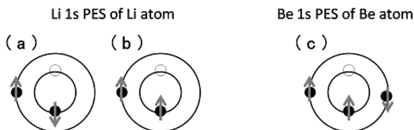
Fig. 4. Schematic illustration of Li 1s PES of Li atom and Be 1s PES of Be atom. Li atom has the open outer shell, while Be the closed outer shell. Due to the reason, Li has two possible final states [(a) and (b)], but Be has only one possible final state [(c)]. Closed dots represent the electrons and the open dots the photoholes, respectively. Arrows signify the electron spins.
