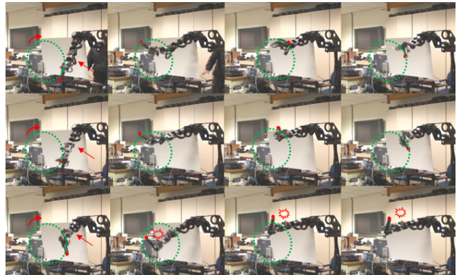
Fig. 7. Snapshots of the experimental results for the 7-DOF robotic arm with respect to the circular motion when sensory feedback of the neural oscillators was turned off.
