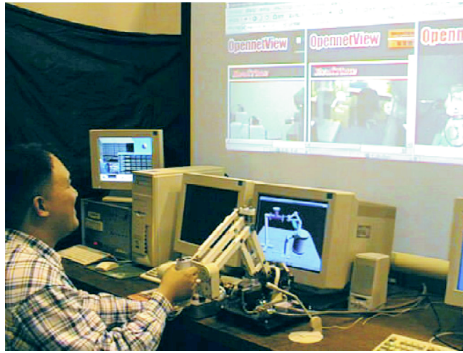
Figure 5: Operator's master control station in AIST.
