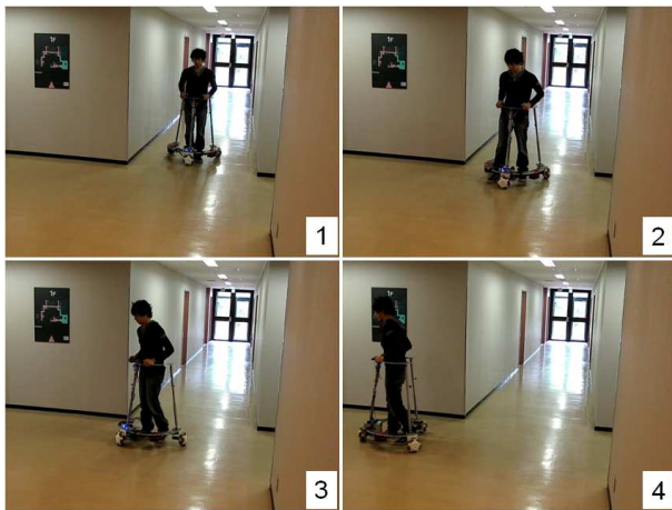
Fig. 14. Forward movement of JARoW around a corner
